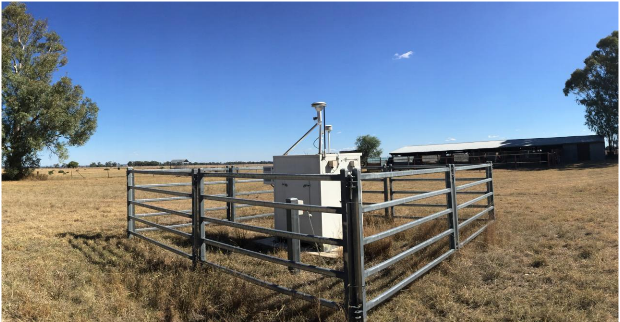
Figure 1: TEOM installed at Flixton property
